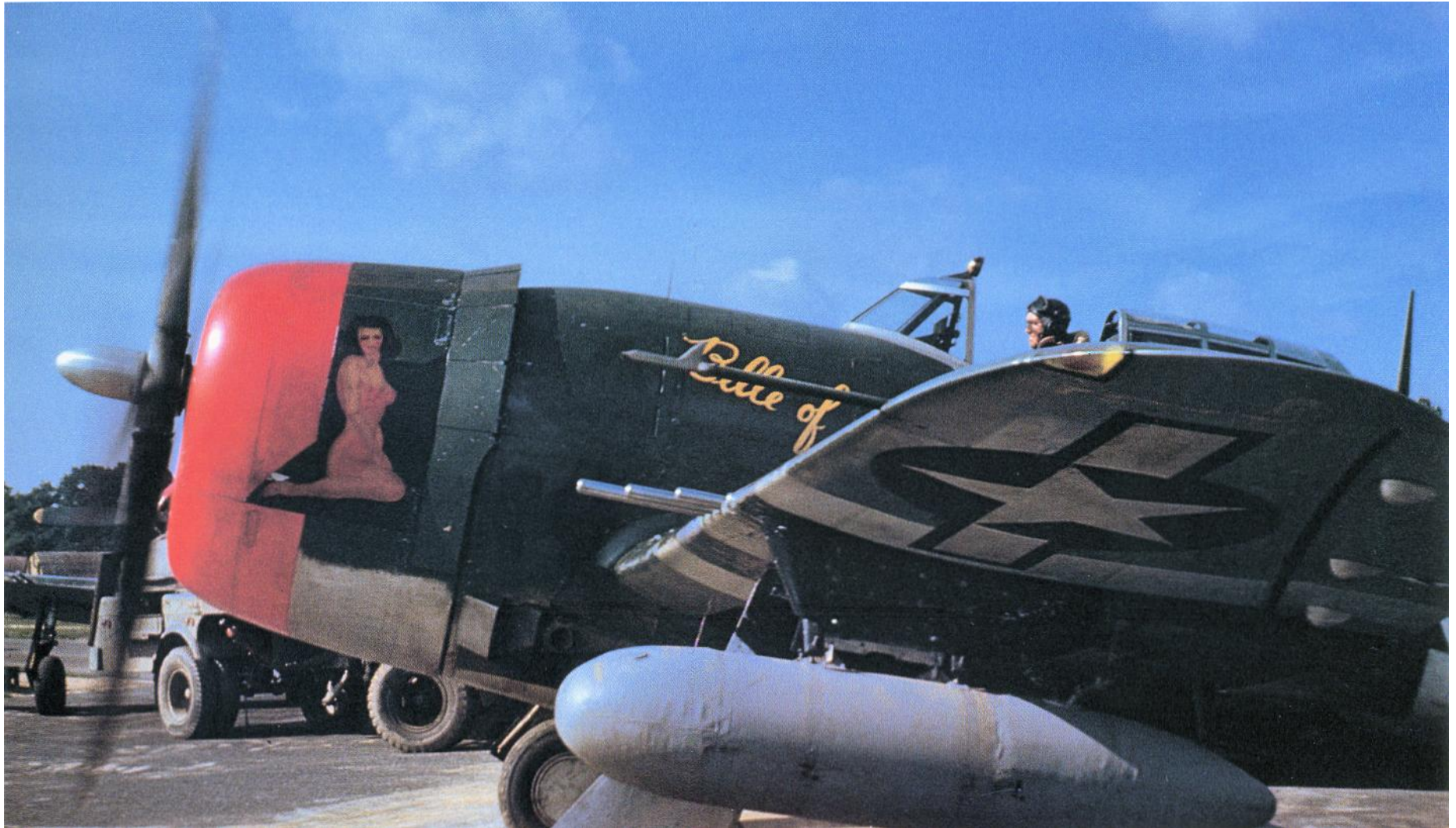
Side view of "Belle". Confirmation of 40 inch (Freeman Type 4) Star and Bar under the port wing. It appears that the Star and Bar may have been repainted. Wing pylon is painted black. Note the undercarriage leg cover only has black portion of invasion stripes applied. The rest of the cover is unpainted (NMF).
